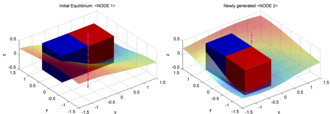
**Figure 4. First reconfiguration example: multibody system equilibria at two nodes in the reconfiguration graph. The dashed line indicates the rotation axis of a revolute joint. The shaded surface's height shows the potential energy as a function of  $x$  and  $y$  position of the bodies. See text for full description.**
