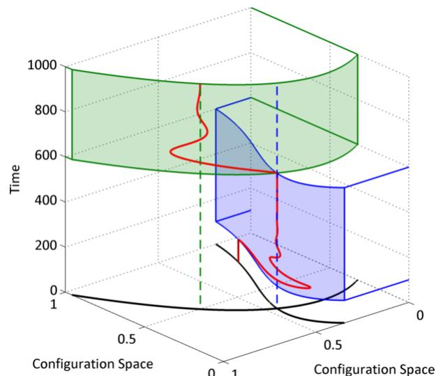
**Figure 1. Sample time history of the system from Figure 2. The control input changes at  $t = 100$  s and again at  $t = 600$  s, triggering discrete transitions in the hybrid automaton.**
