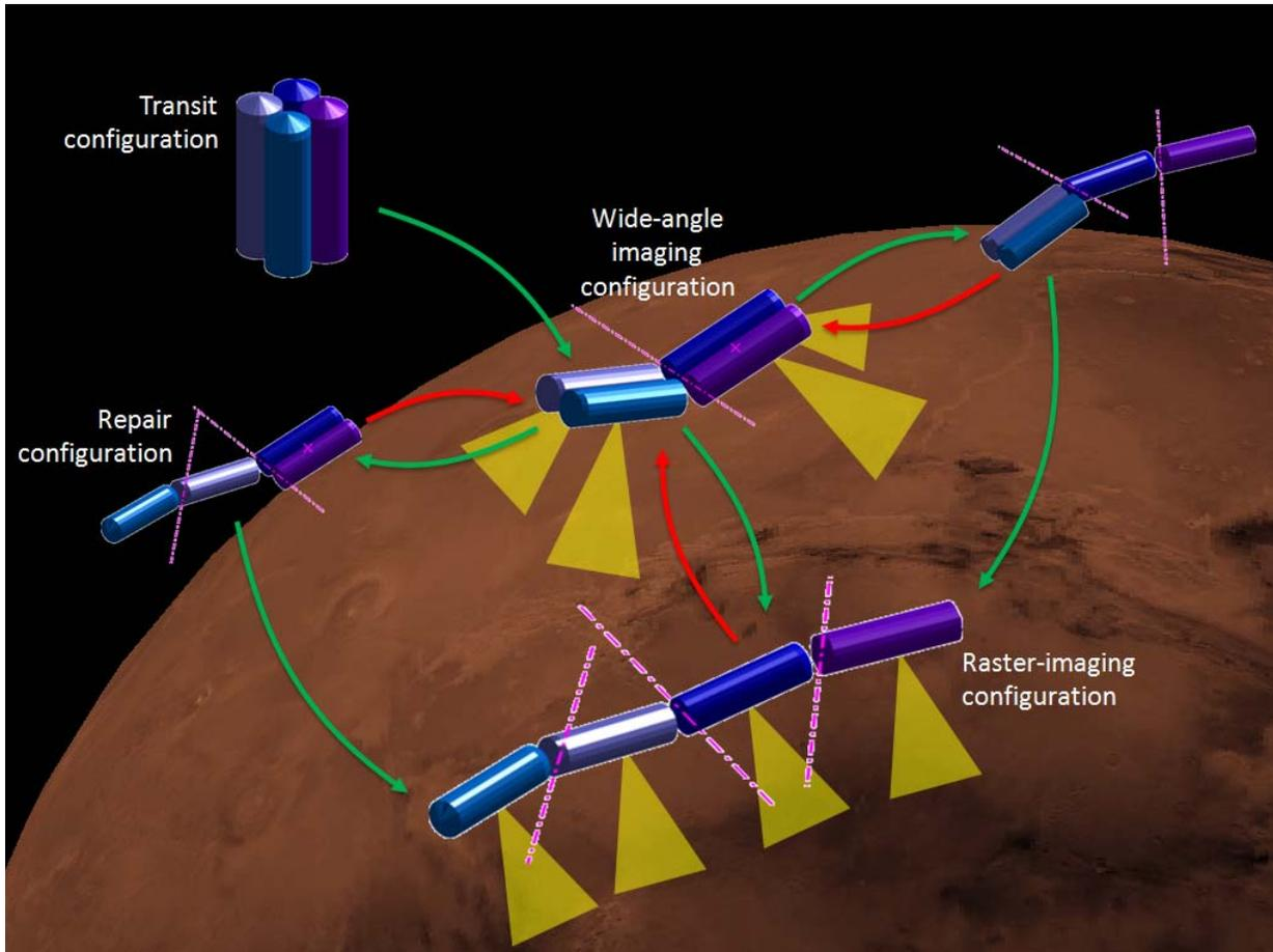
**Figure 7. Partial reconfiguration graph for a hypothetical planetary imaging mission. Dashed lines indicate hinges. See text for full description.**
