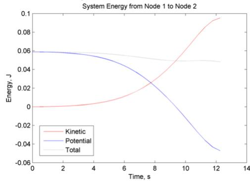
Figure 5. System energy as a function of time.
