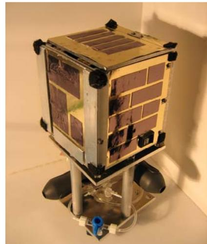
**Figure 8. Air-levitated, CubeSat-sized laboratory demonstration unit.**
