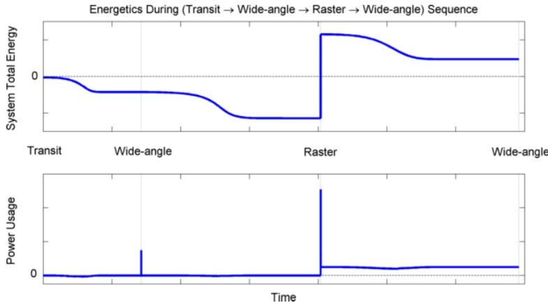
**Figure 9. Qualitative total system energy and power usage for a sample reconfiguration sequence of the planetary imaging mission. See text for full description.**
