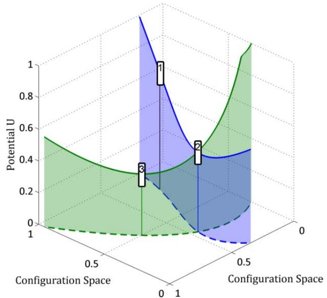
**Figure 2. Illustration of the stepwise passive reconfiguration concept in a system with two possible degrees of freedom augmented with potentials.**
